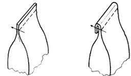
Fold-over closure manually by operator or by additional bag feed-in device with bag-top fold-over device
