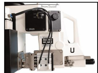
**Advantage:** Reliable trimming of thread chain with or without filler cord (respectively crepe tape).
