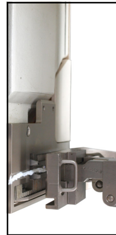
Fold-over closure manually by operator or by additional bag feed-in device with bag-top fold-over device
